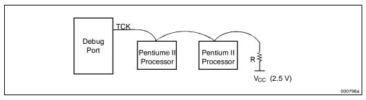
Figure 13-5. TCK with Daisy Chain Configuration
