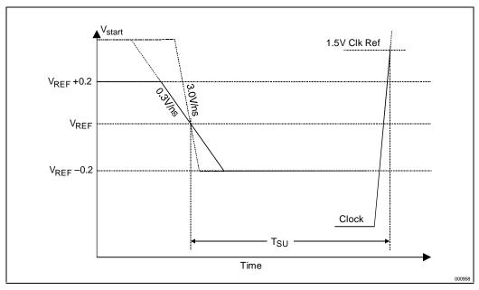
Figure 8-12. Standard Input Hi-to-Lo Waveform for Characterizing Receiver Setup Time
