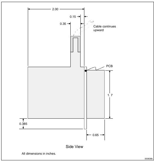
Figure 13-13. Pentium® II Processor Integration Tool Mechanical Keep Out Volume— Side View
