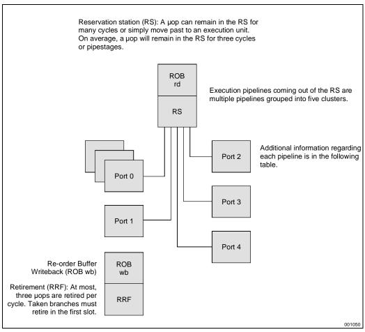
Figure 2-9. Out-of-Order Core and Retirement Pipeline
