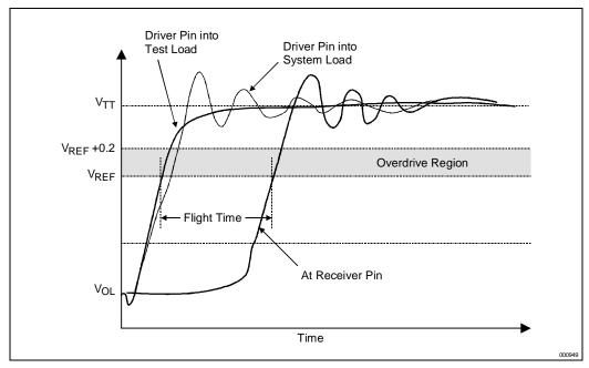
Figure 8-5. Measuring Nominal Flight Time
