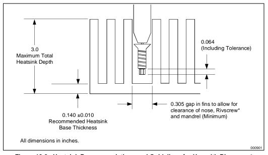
Figure 10-9. Heatsink Recommendations and Guidelines for Use with Rivscrews\*
