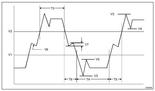
Figure 9-1. BCLK, TCK PICCLK Generic Clock Waveform at the Processor Edge Fingers
