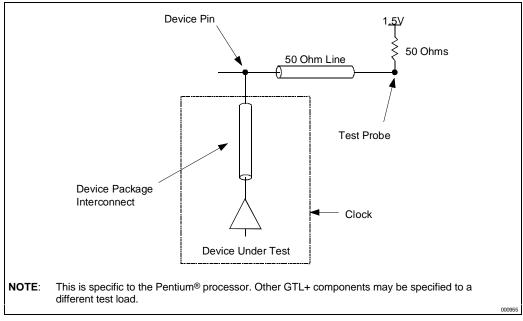
Figure 8-9. Test Load for Measuring Output AC Timings
