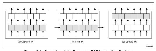
Figure 6-4. Operation of the Processor TAP Instruction Register
