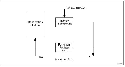
Figure 2-6. Inside the Retire Unit
