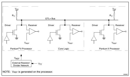
Figure 8-1. Example Terminated Bus with GTL+ Transceivers
