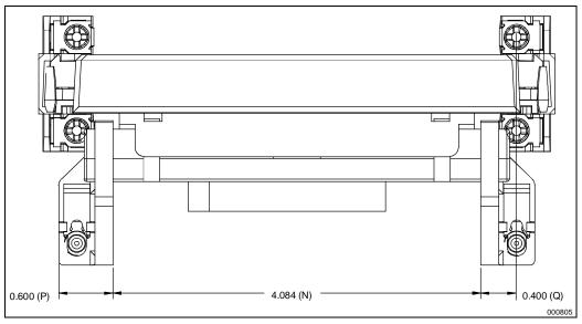
Figure 12-7. Top View Space Requirements for Boxed Processor Fan/Heatsink Supports
