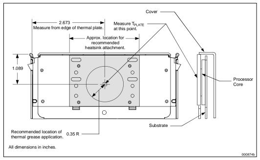
Figure 10-2. Processor Thermal Plate Temperature Measurement Location
