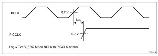
Figure 7-9. FRC Mode BCLK to PICCLK Timing
