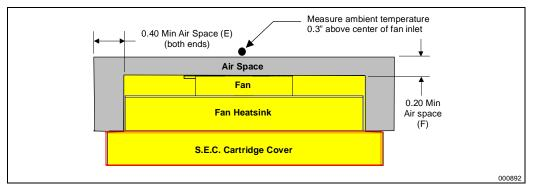
Figure 12-4. Top View Space Requirements for the Boxed Processor
