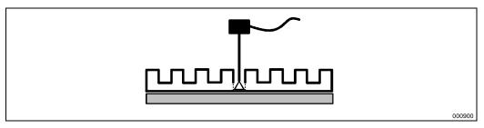
Figure 10-4. Technique for Measuring T<sub>PLATE</sub> with 90° Angle Attachment
