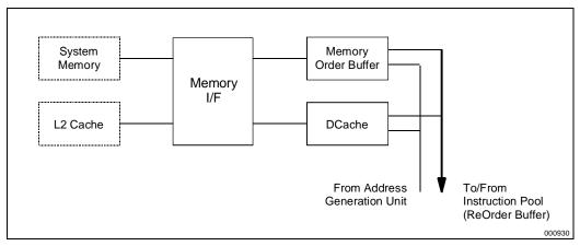
Figure 2-7. Inside the Bus Interface Unit
