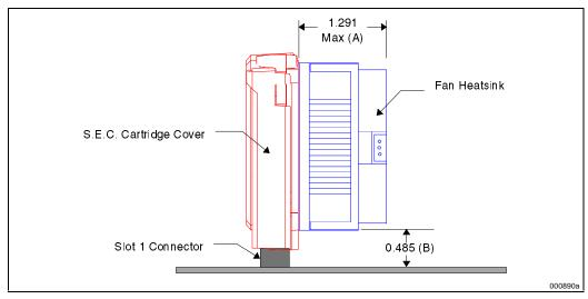
Figure 12-2. Side View Space Requirements for the Boxed Processor (Fan/heatsink supports not shown)
