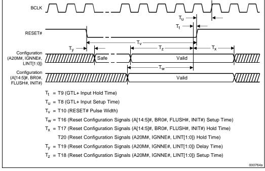
Figure 7-10. System Bus Reset and Configuration Timings
