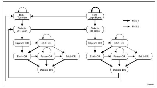
Figure 6-2. TAP Controller Finite State Machine
