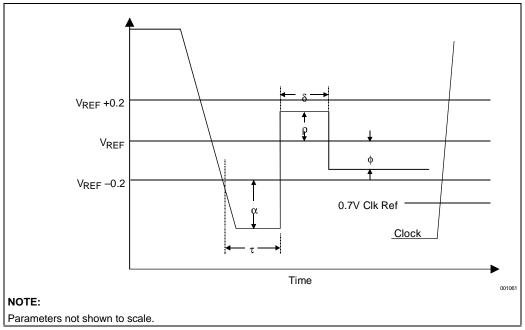
Figure 8-4. Standard Input Hi-to-Lo Waveform for Characterizing Receiver Ringback Tolerance
