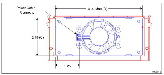
Figure 12-3. Front View Space Requirements for the Boxed Processor
