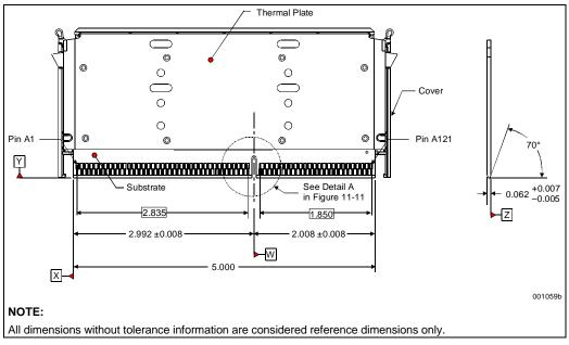
Figure 11-9. S.E.C. Cartridge Substrate Dimensions (Skirt not shown for clarity)
