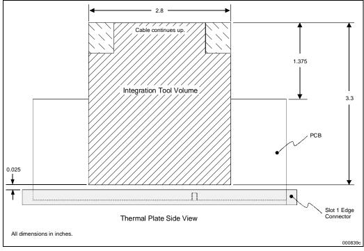
Figure 13-11. Pentium® II Processor Integration Tool Mechanical Keep Out Volume— Thermal Plate Side View
