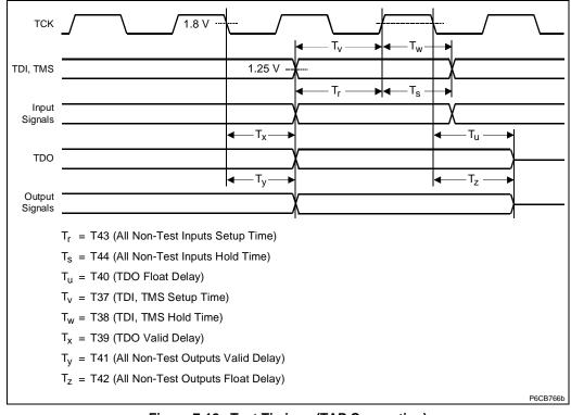
Figure 7-12. Test Timings (TAP Connection)
