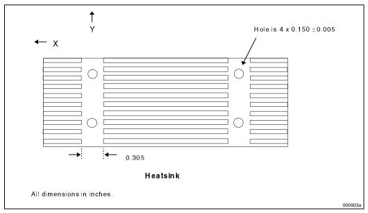
Figure 10-11. General Rivscrew\* Heatsink Mechanical Recommendations
