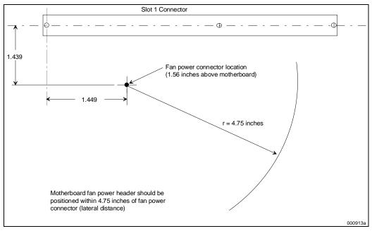
Figure 12-9. Recommended Motherboard Power Header Placement Relative to Fan Power Connector and Slot 1
