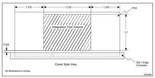
Figure 13-12. Pentium® II Processor Integration Tool Mechanical Keep Out Volume—Cover Side View
