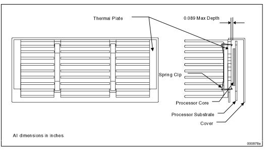
Figure 10-8. Processor with an Example Full Height Heatsink Attached using Spring Clips
