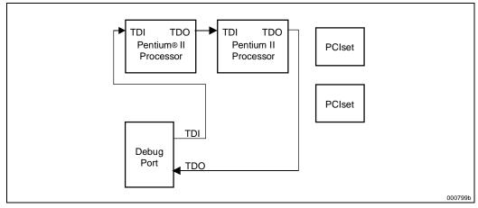
Figure 13-9. Processor System where Boundary Scan is Not Used
