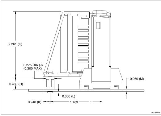
Figure 12-6. Side View Space Requirements for Boxed Processor Fan/Heatsink Supports
