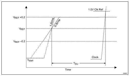
Figure 8-11. Standard Input Lo-to-Hi Waveform for Characterizing Receiver Setup Time
