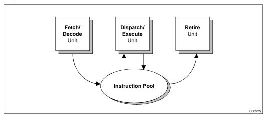
Figure 2-1. Three Engines Communicating Using an Instruction Pool
