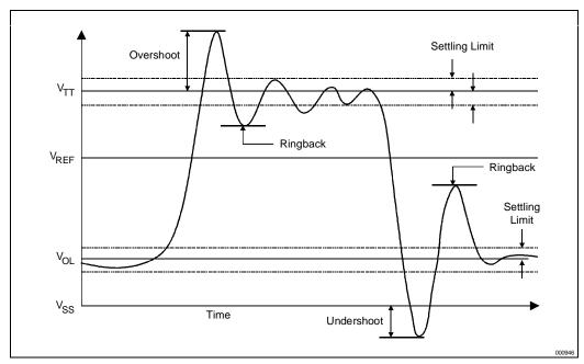
Figure 8-2. Receiver Waveform Showing Signal Quality Parameters
