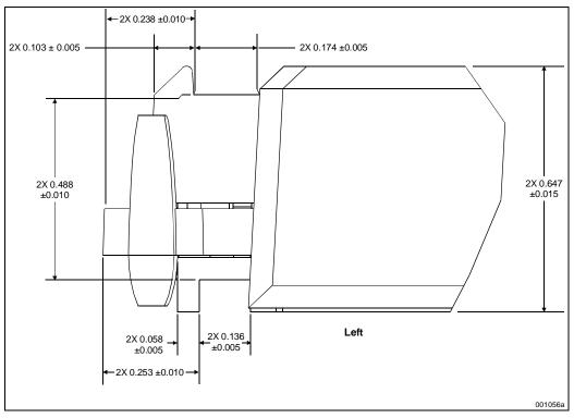
Figure 11-7. S.E.C. Cartridge Latch Arm, Thermal Plate Lug and Cover Lug Dimensions
