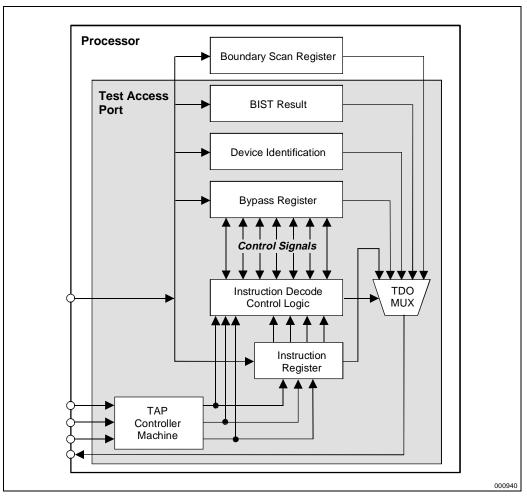
Figure 6-1. Simplified Block Diagram of Processor TAP Logic
