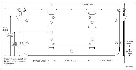
Figure 11-4. S.E.C. Cartridge Thermal Plate Side Dimensions
