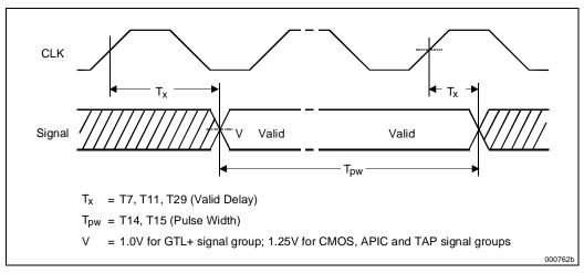
Figure 7-7. System Bus Valid Delay Timings
