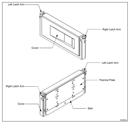
Figure 11-1. S.E.C. Cartridge—Thermal Plate and Cover Side Views
