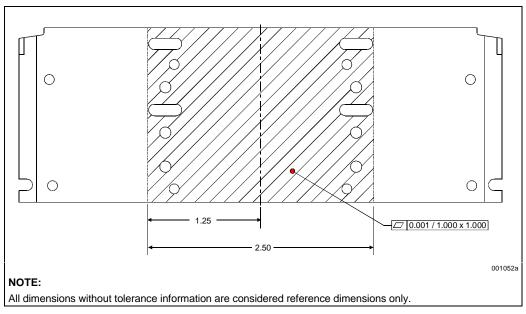
Figure 11-5. S.E.C. Cartridge Thermal Plate Flatness Dimensions
