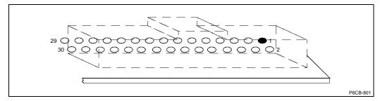
Figure 13-8. Hole Positioning for Connector on Thermal Plate Side of Circuit Board
