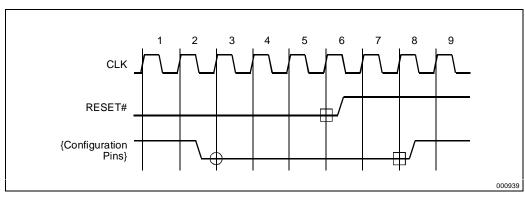
Figure 5-1. Hardware Configuration Signal Sampling
