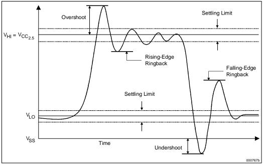
Figure 9-2. Non-GTL+ Overshoot/Undershoot and Ringback Tolerance
