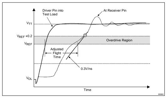
Figure 8-6. Flight Time of a Rising Edge Slower than 0.3V/ns
