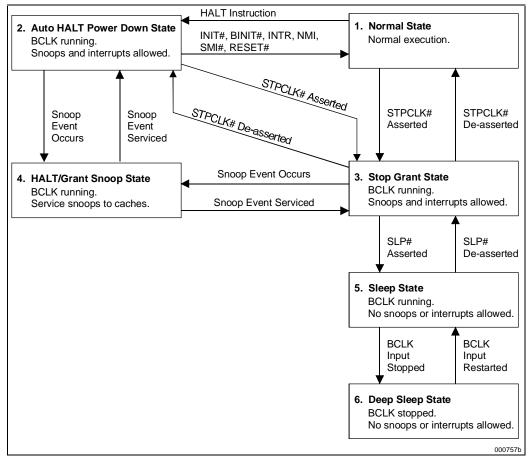
Figure 7-2. Stop Clock State Machine
