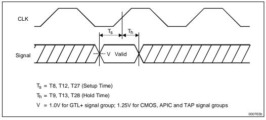
Figure 7-8. System Bus Setup and Hold Timings
