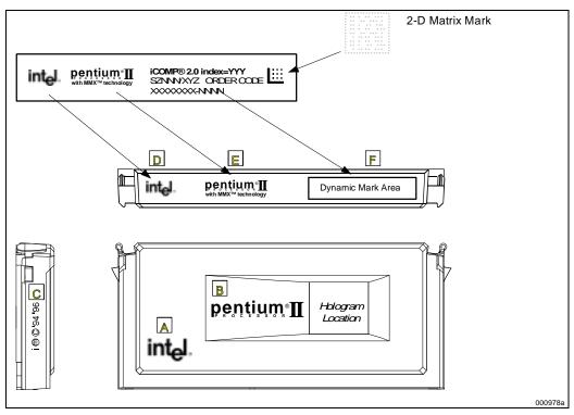
Figure 11-12. S.E.C. Cartridge Mark Locations (Processor Markings)
