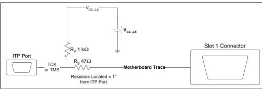
Figure 13-3. TCK/TMS with Series and Parallel Termination, Single Processor Configuration
