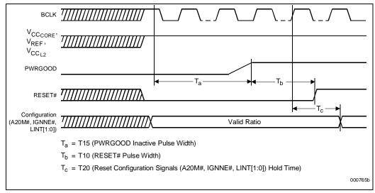
Figure 7-11. Power-On Reset and Configuration Timings
