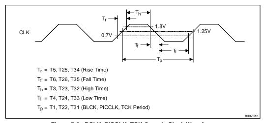
Figure 7-6. BCLK, PICCLK, TCK Generic Clock Waveform
