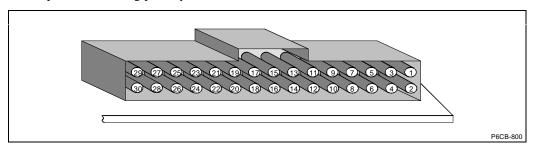
Figure 13-7. Debug Port Connector on Thermal Plate Side of Circuit Board
