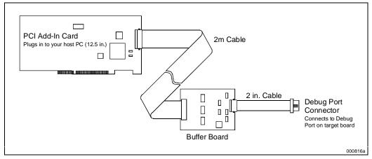
Figure 13-1. Hardware Components of the ITP
