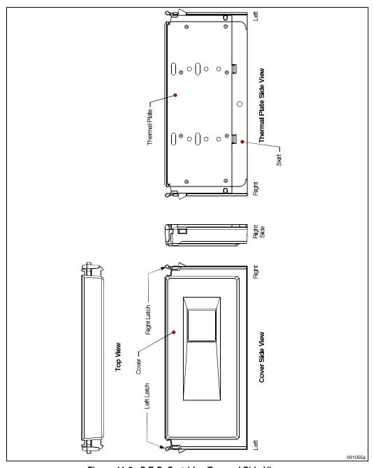
Figure 11-2. S.E.C. Cartridge Top and Side Views
