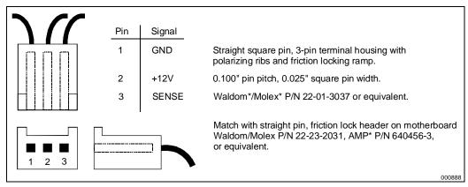
Figure 12-8. Boxed Processor Fan/Heatsink Power Cable Connector Description
