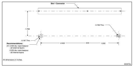
Figure 12-5. Heatsink Support Hole Locations and Sizes
