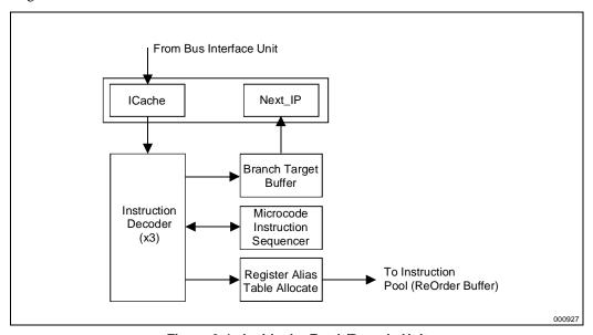
Figure 2-4. Inside the Fetch/Decode Unit
