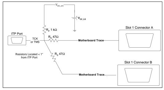
Figure 13-4. TCK/TMS with Daisy Chain Configuration, 2-Way MP Configuration
