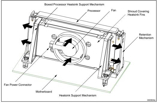
Figure 12-1. Conceptual Boxed Pentium® II Processor in Retention Mechanism
