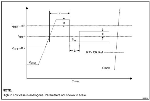
Figure 8-3. Low to High GTL+ Receiver Ringback Tolerance
