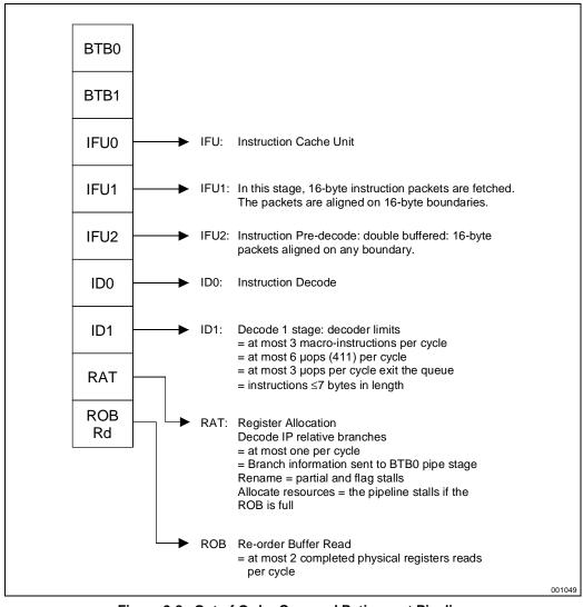
Figure 2-8. Out of Order Core and Retirement Pipeline
