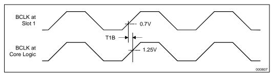
Figure 7-5. BCLK to Core Logic Offset
