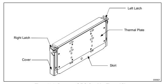
Figure 10-1. Processor S.E.C. Cartridge Thermal Plate
