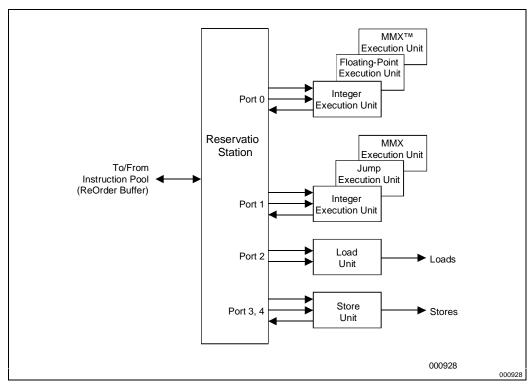
Figure 2-5. Inside the Dispatch/Execute Unit
