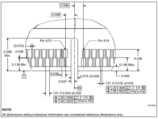
Figure 11-11. S.E.C. Cartridge Substrate—Detail A
