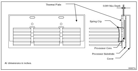
Figure 10-7. Processor with an Example Low Profile Heatsink Attached using Spring Clips
