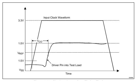
Figure 8-10. Clock to Output Data Timing (T<sub>CO</sub>)
