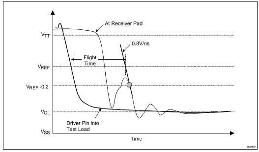
Figure 8-8. Extrapolated Flight Time of a Non-Monotonic Falling Edge
