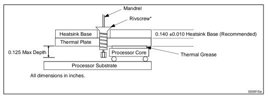
Figure 10-10. Heatsink, Rivscrew\* and Thermal Plate Recommendations and Guidelines
