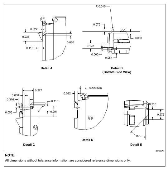
Figure 11-8. S.E.C. Cartridge Latch Arm, Cover and Thermal Plate Detail Dimensions
