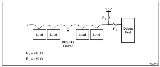
Figure 13-2. GTL+ Signal Termination
