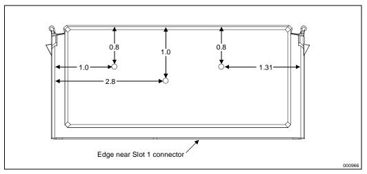
Figure 10-5. Guideline Locations for Cover Temperature (T<sub>COVER</sub>)
