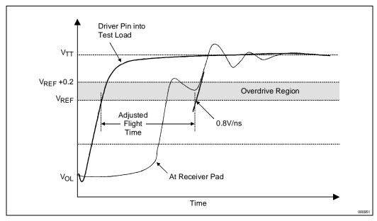
Figure 8-7. Extrapolated Flight Time of a Non-Monotonic Rising Edge
