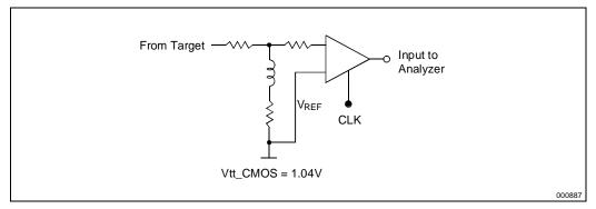
Figure 13-10. LAI Probe Input Circuit
