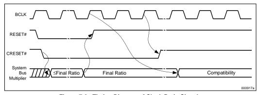
Figure 7-3. Timing Diagram of Clock Ratio Signals
