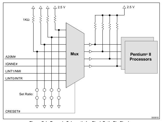
Figure 7-4. Example Schematic for Clock Ratio Pin Sharing
