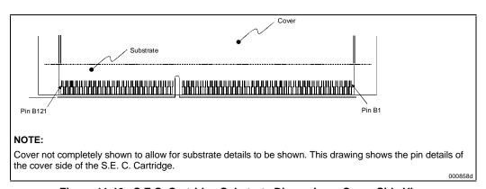
Figure 11-10. S.E.C. Cartridge Substrate Dimensions, Cover Side View
